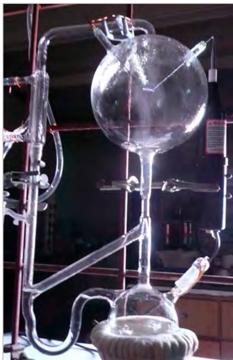
The "volcanic" apparatus showing the jet of steam into the spark flask. (Courtesy David Brigg BBC Scotland)
